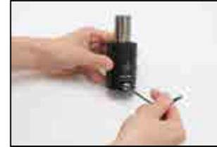
2. Use a degassing jig (LSTL-GL) to discharge gas.
