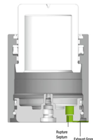
The rupture septum on the base of the gas spring will break should the internal pressure exceed the specified value. Consequently, the internal nitrogen gas will be exhausted via the exhaust groove. You can judge the OPAS has worked if the rupture septum is open.
