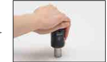
4. Remove the gas charge valve with the special screwdriver (LSTL-VD).
