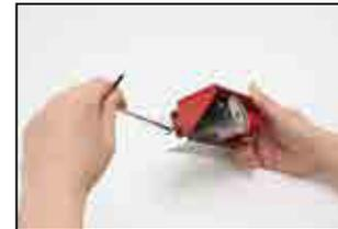
9. Install the conversion adapter the control panel insertion port.
