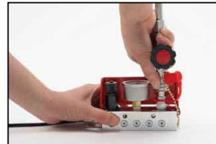
23. Loosen the valve on the gas tank side to release the residual pressure in the hose.
