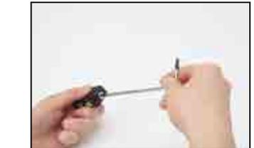
8. Remove the control panel cap with hexagon wrench.
